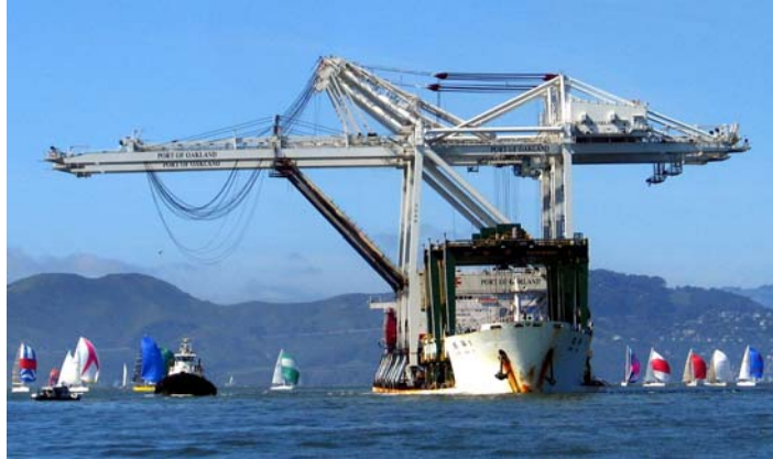
A shore-based gantry crane similar in size to the one being built for Esperance Port is delivered to the Port of Oakland in San Francisco Bay aboard a dedicated ZPMC delivery vessel.
